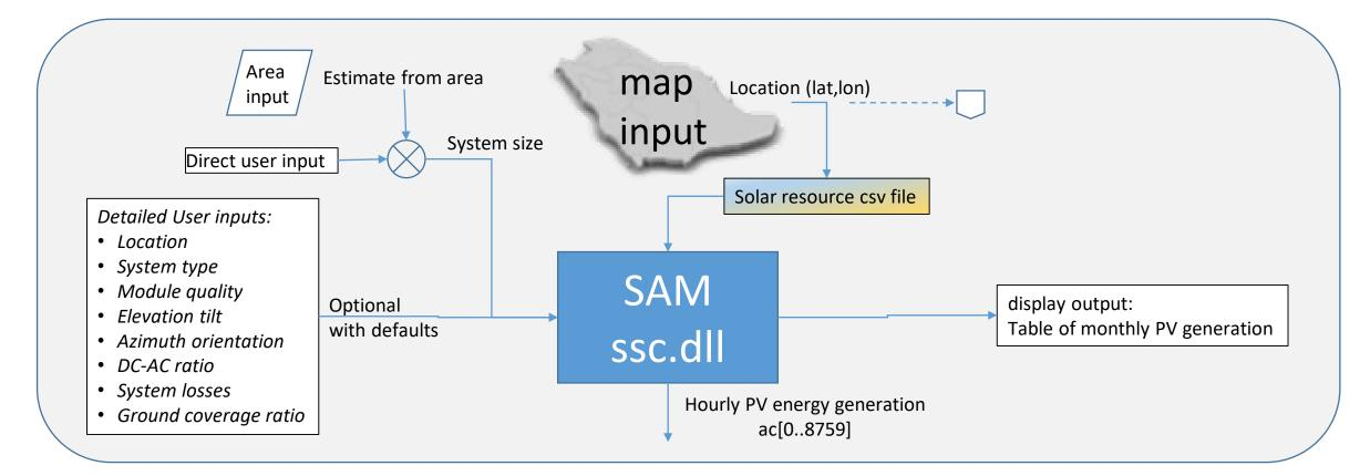
The solar calculator is directly using the open-source System Advisor Model (SAM) developed and maintained by the US National Renewable Energy Laboratory (NREL)
