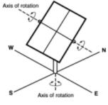
Two-axis tracking PV array
