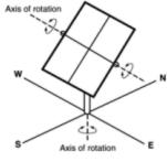
Two-axis tracking PV array
