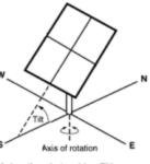
Azimuth-axis tracking PV array
