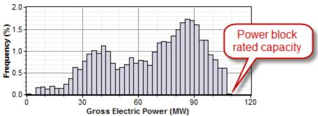
For the same system with a solar multiple chosen to minimize LCOE (in this example SM=1.5), the power cycle generates electricity at or slightly above its rated capacity almost 15% of the time:
