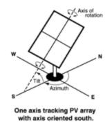
For 1-axis tracking, PVWatts models self shading based on the ground coverage ratio (GCR).
