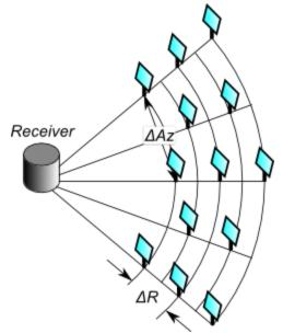
The initial spacing between heliostats in a row is a distance twice the width of a heliostat. As the radial position of the rows increases, so too does the spacing between heliostats as they maintain their position along an azimuthal line. Spacing continues to increase until the distance between heliostats meets or exceeds 2  $\frac{2}{3}$  times the heliostat width. Spacing then resets to the original factor of 2 times the width.
