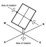
Two-axis tracking PV array
