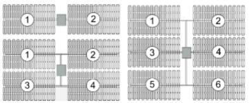
The number of field subsections determine the location and shape of header piping that delivers heat transfer fluid to the power block, which affects the heat loss calculation.
