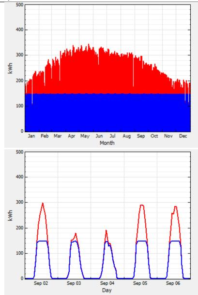
• Inverter output less than 75 percent of inverter rated capacity. SAM compares the inverter's maximum AC output to the total inverter AC capacity and displays a simulation warning if the inverter's maximum AC output is less than 75% of the total inverter rated AC capacity.
