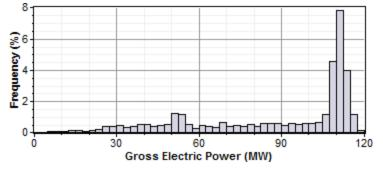
Adding thermal storage to the system changes the optimal solar multiple, and increases the amount of time that the power cycle operates at its rated capacity. In this example, the optimal storage capacity (full load hours of TES) is 3 hours with SM=1.75, and the power cycle operates at or over its rated capacity over 20% of the time:
