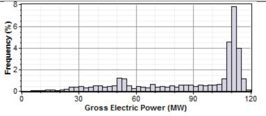
Adding thermal storage to the system changes the optimal solar multiple, and increases the amount of time that the power cycle operates at its rated capacity. In this example, the optimal storage capacity (full load hours of TES) is 3 hours with SM=1.75, and the power cycle operates at or over its rated capacity over 20% of the time:
