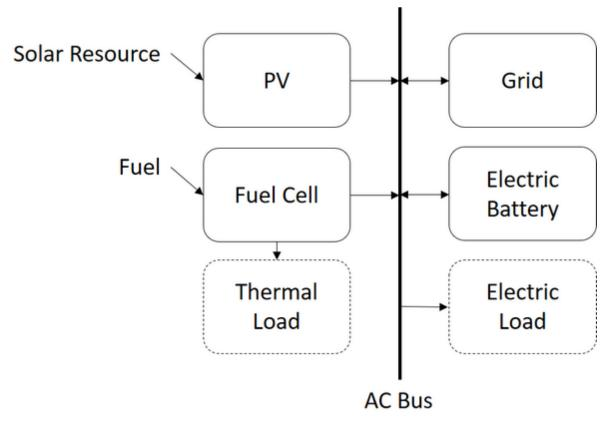
The fuel cell performance model uses the following input pages to describe the components of a grid-connected tri-generation system:
