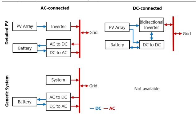
Figure 1: Front-of-meter Battery Configurations
