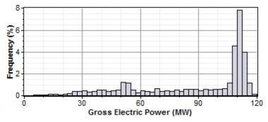
Adding thermal storage to the system changes the optimal solar multiple, and increases the amount of time that the power block operates at its rated capacity. In this example, the optimal storage capacity (full load hours of TES) is 3 hours with SM=1.75, and the power block operates at or over its rated capacity over 20% of the time:
