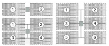
The number of field subsections determine the location and shape of header piping that delivers heat transfer fluid to the power block, which affects the heat loss calculation.
