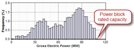
For the same system with a solar multiple chosen to minimize LCOE (in this example SM=1.5), the power block generates electricity at or slightly above its rated capacity almost 15% of the time:
