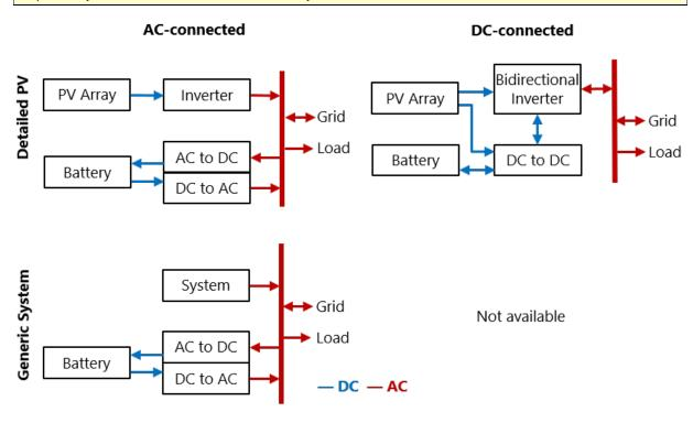
Figure 1: Behind-the-meter Battery Configurations
