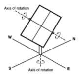
Two-axis tracking PV array
