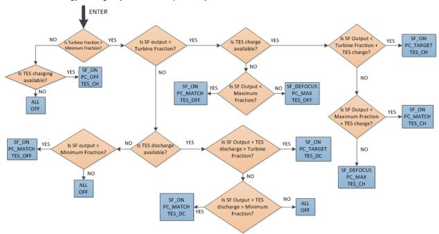
When you run a simulation without enabling optimization, SAM attempts to operate the system so that the power cycle output matches the dispatch schedule you define. If the turbine dispatch fraction for a given time step is greater than the minimum turbine fraction and the storage system is full, it will dispatch energy to the power cycle up to the turbine output fraction for that time step, and defocus the field if the field thermal power output exceeds the amount required.
