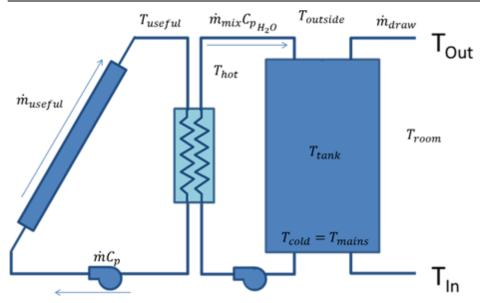
The specific equations solved depend on whether useful solar energy is being collected or not. Below is a system diagram for when energy is being collected.
