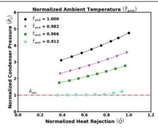
In hybrid cooling, a wet-cooling system and dry-cooling share the heat rejection load. Although there are many possible theoretical configurations of hybrid cooling systems, SAM only allows a parallel cooling option.
