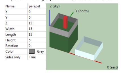
Examples of Box Shading Objects with Properties and in 3D Scene View
