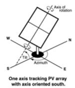
For 1-axis tracking, PVWatts models self shading based on the ground coverage ratio (GCR).
