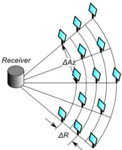
The initial spacing between heliostats in a row is a distance twice the width of a heliostat. As the radial position of the rows increases, so too does the spacing between heliostats as they maintain their position along an azimuthal line. Spacing continues to increase until the distance between heliostats meets or exceeds  $2 \frac{2}{3}$  times the heliostat width. Spacing then resets to the original factor of 2 times the width.
