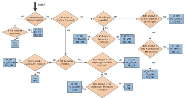
When you run a simulation without enabling optimization, SAM attempts to operate the system so that the power cycle output matches the dispatch schedule you define. If the turbine dispatch fraction for a given time step is greater than the minimum turbine fraction and the storage system is full, it will dispatch energy
