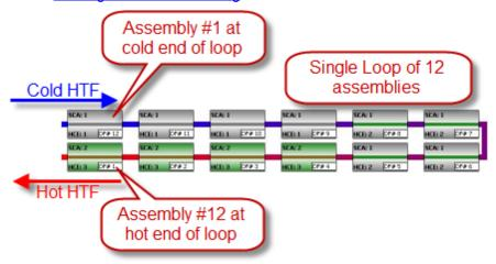
The color of the rectangle and SCA number indicates the collector type of each assembly. Similarly, the color of the line representing the receiver and the HCE number indicates the receiver type. The "DF" number indicates the collector defocusing order:
