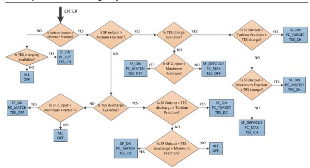
When you run a simulation without enabling optimization, SAM attempts to operate the system so that the power cycle output matches the dispatch schedule you define. If the turbine dispatch fraction for a given time step is greater than the minimum turbine fraction and the storage system is full, it will dispatch energy to the power cycle up to the turbine output fraction for that time step, and defocus the field if the field thermal power output exceeds the amount required.
