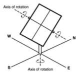
Two-axis tracking PV array
