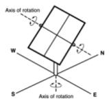
Two-axis tracking PV array
