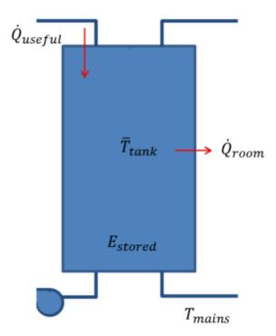
During solar collection, the tank is assumed to be fully mixed. This assumption is made because hot water continually is entering the top of the tank and mixing with cooler water underneath. A simple energy balance is performed on the tank to solve for the mean tank temperature each hour. Note that energy is added from the solar collector loop, energy is lost to the environment, mass enters the tank at the mains temperature
