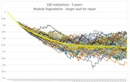
20% module degradation rate, 5-year analysis with 100 realizations on base 4 kW (24 module) system.
