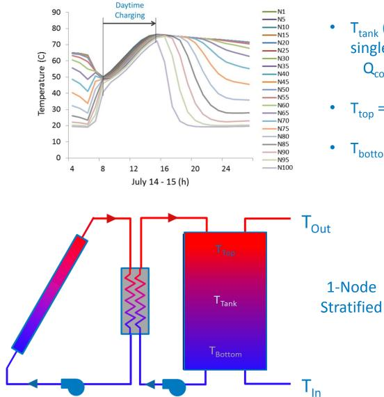
T<sub>tank</sub> (average tank temperature ) single-node energy balance: Q<sub>coll,hx</sub> + Q<sub>room</sub> + Q<sub>cold</sub>
